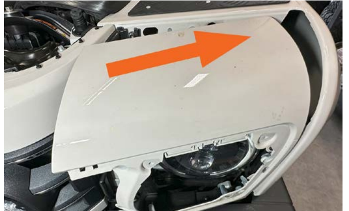
42. Come in at an angle when installing the painted headlight panel.
