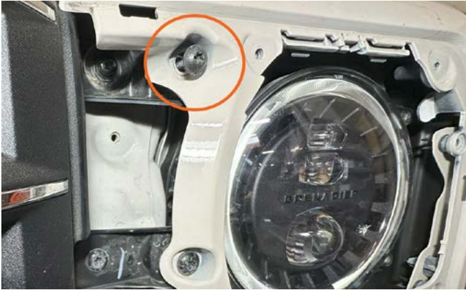
45. The extra-long T40 bolt goes in upper headlight panel.
