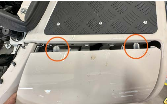
43. Now line up panel pins with the holes in fender. When lined up, push panel into place.
