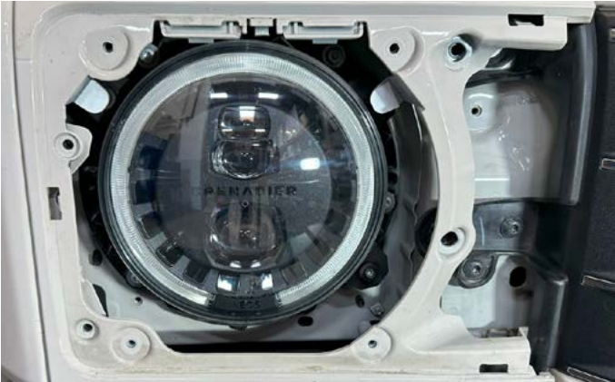
7. With the four headlight panel screws removed, pull out panel starting from the lower fender corner.
