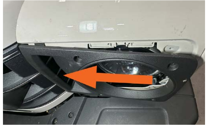
46. Come in at an angle when installing the headlight bezel then snap bezel into place.
