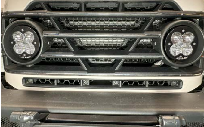
41. With both bezels installed, re-install the 4 lower grille bolts from step 13. Re-assemble grille and headlight panels using factory hardware. Refer back to steps 1-13.
