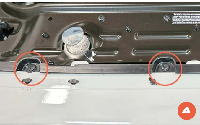
11 A/B. Locate the 4 upper grille retainer clips.
