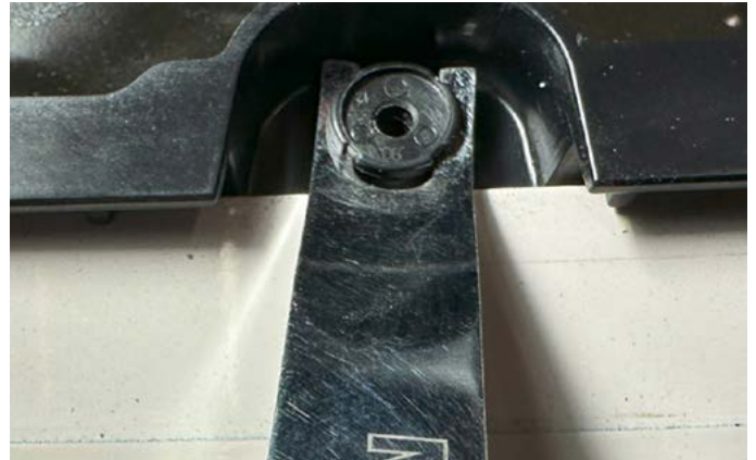
13. Then remove the remaining clip using a clip removal tool. Remove all 4 retaining clips.
