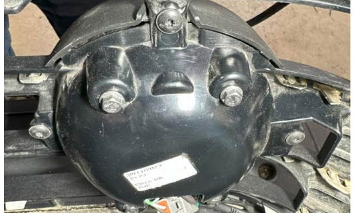
40. Re-install the factory lamp bezel using the factory screws.
