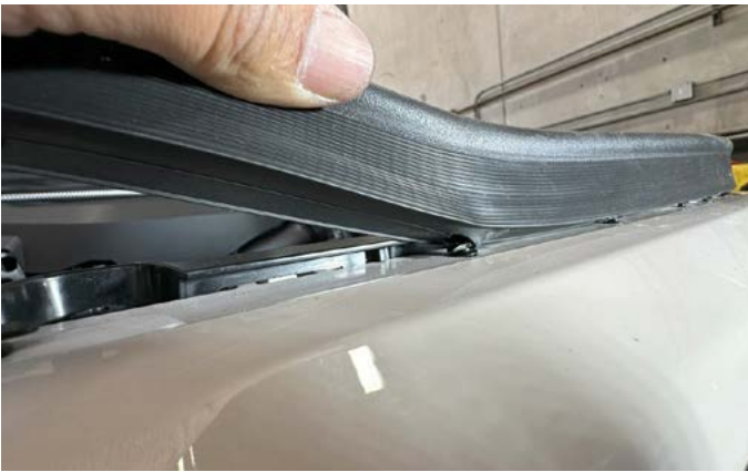
47. Start the weatherstrip installation from one end and work around until all t-clips are re-attached. Slide weatherstrip onto one end of t-clip then stretch weatherstrip and let it snap back until the clip is completely inserted in weatherstrip.
