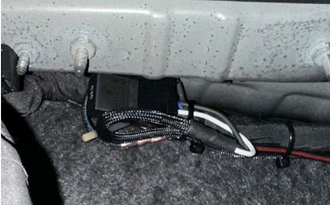
39. Zip tie the relay assembly to the factory wire harness as shown.
