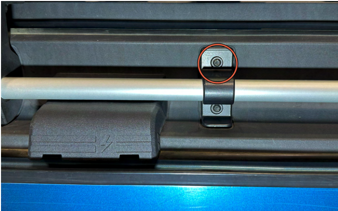
5. Use a T30 Torx bit to remove the upper grab handle bolt.
